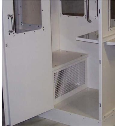
**Air Exchange Rate** - The volume of air being exhausted from the chamber is 140 CFM. This volume of exhaust means that the air within the chamber is exchanged in excess of 150 times per hour.
